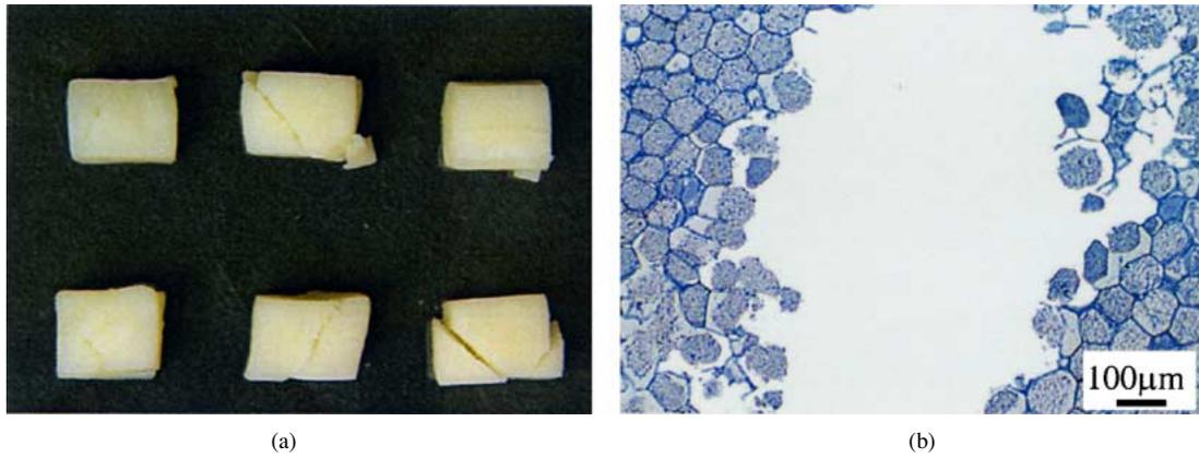
Figure 2 Chinese water chestnut compressed at 500 mm/min to 25% strain: (a) showing shear, brittle fractures and (b) fracture path through cells.
