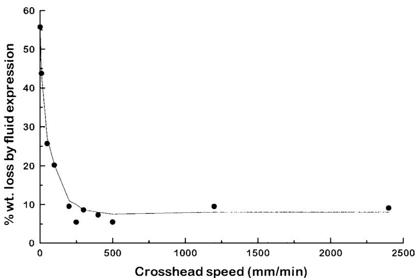
Figure 7 The dependence of the fluid expression during compression from processed Chinese water chestnut tissue on strain rate.
