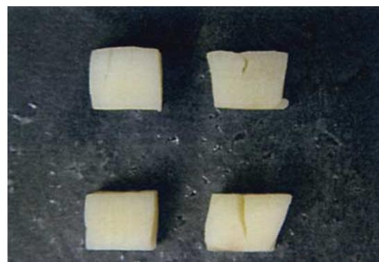
Figure 5 Chinese water chestnut compressed at 100 mm/min to 25% strain—tensile fracture apparent.
