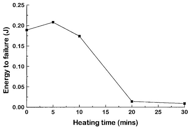
Figure 14 The variation in energy to failure, during compression at 500 mm/min, with heating time.
