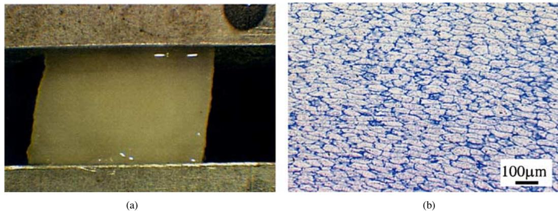
Figure 4 Chinese water chestnut compressed at 2 mm/min to: (a) 25% strain—fluid expression, no barrelling and (b) 80% strain—failure by cell wall buckling.
