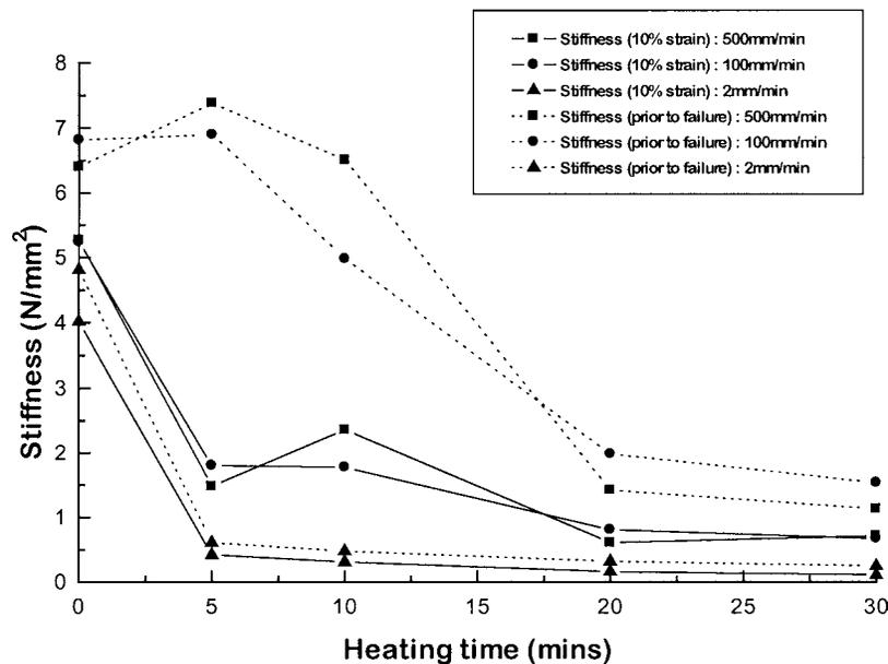
Figure 12 The variation in carrot tissue stiffness (on initial deformation & prior to failure) with heating time, at a range of strain rates.
