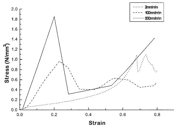
Figure 1 The dependence of the compressive mechanical behaviour of processed Chinese water chestnut tissue on strain rate.
