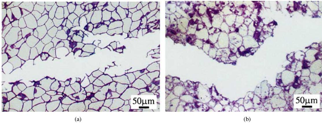
Figure 11 Carrot compressed at 500 mm/min to 25% strain: (a) Raw carrot; brittle fracture through cells and (b) Carrot heated for 30 min; fracture occurs between cells.
