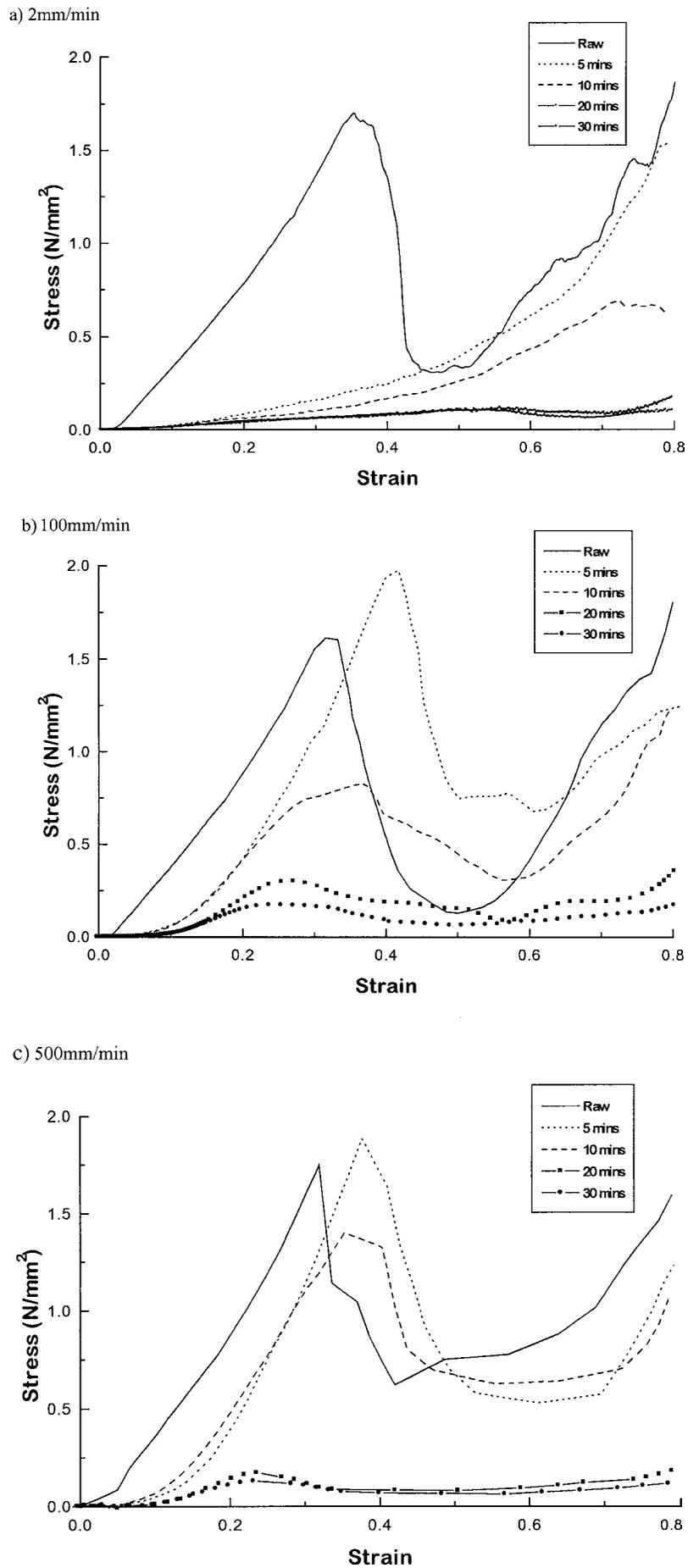
Figure 10 The mechanical behaviour of carrot tissue, subjected to a range of heating times, compressed at: (a) 2 mm/min, (b) 100 mm/min and (c) 500 mm/min.
