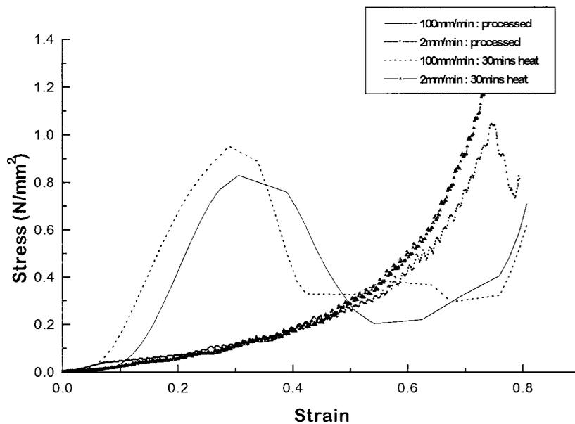
Figure 9 Comparison of the mechanical behaviour of processed Chinese water chestnut tissue and tissue heated at 100°C for 30 min.
