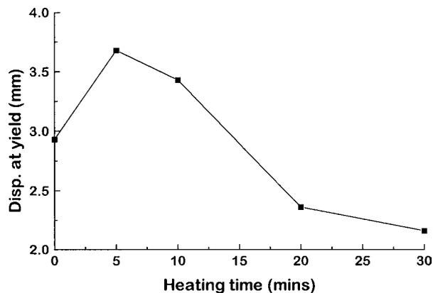
Figure 15 The variation in displacement at yield, during compression at 500 mm/min, with heating time.
