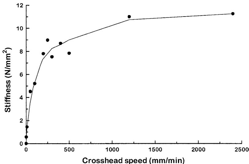
Figure 6 The dependence of the stiffness of processed Chinese water chestnut tissue on strain rate.
