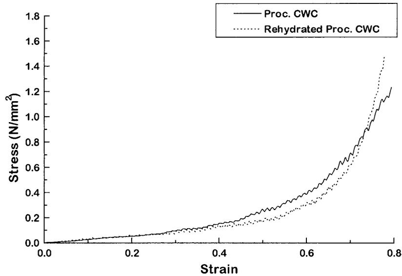
Figure 8 Comparison of the mechanical behaviour at low strain rate of processed Chinese water chestnut tissue (CWC) and compressed tissue following immersion in water.
