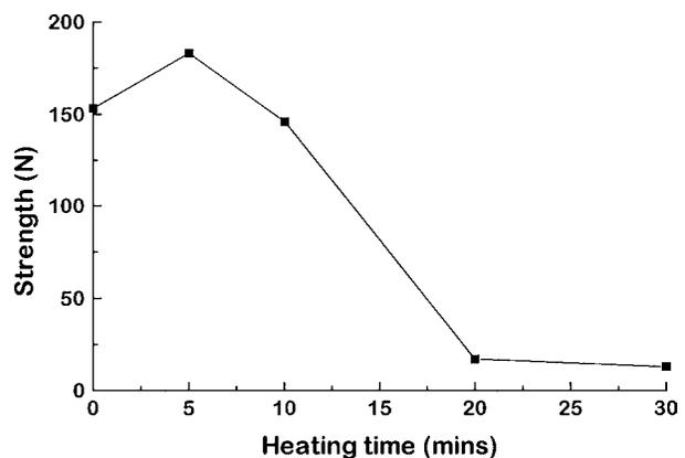
Figure 13 The variation in tissue strength, during compression at 500 mm/min, with heating time.
