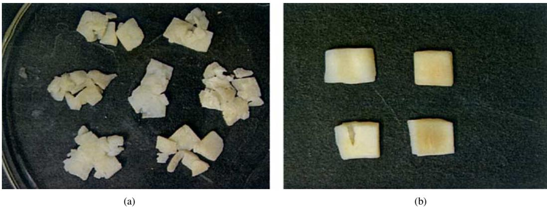
Figure 3 Chinese water chestnut compressed at: (a) 100 mm/min to 80% strain—many fragments formed and (b) 2 mm/min to 80% strain—flattened cube (square) formed, with some fracture occurring at high strain.
